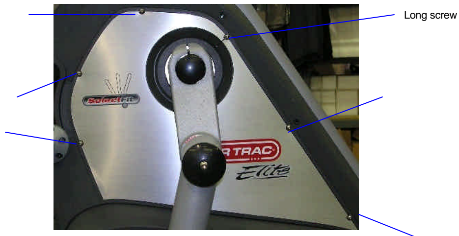
Figure 2 Shroud Access Panel
